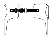
Newport® 3 Bi-Lateral Pelvic Components Adapted for bilateral application. The bilateral model features 2 modular pelvic components predrilled to accept hip joints. Features are described above. Click'n close fastener is standard, chafe and loop is also available.
